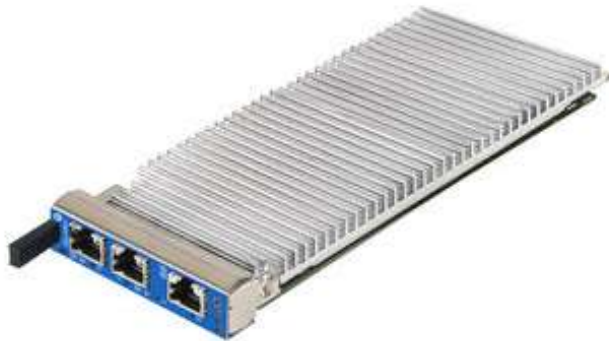
One 1GHz processor under a full-size heatsink
