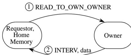
**Figure 3-22. Flush Operation to Local Modified Coherence Granule**
