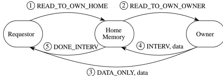
**Figure 3-9. Read-for-Ownership Operation to Remote Modified Coherence Granule**
