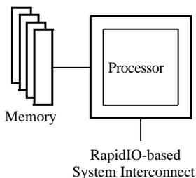
**Figure 2-3. Integrated Processor-Memory Processing Element Example**
