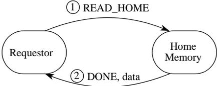
Figure 3-1. Read Operation to Remote Shared Coherence Granule
