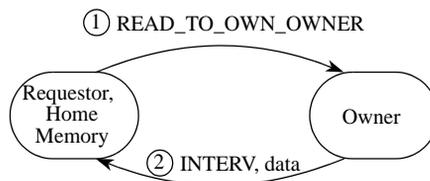
**Figure 3-11. Read-for-Ownership Operation to Local Modified Coherence Granule**
