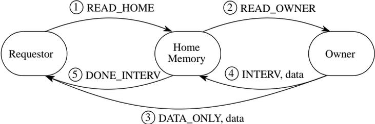
Figure 3-2. Read Operation to Remote Modified Coherence Granule
