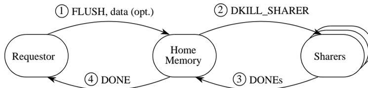
**Figure 3-19. Flush Operation to Remote Shared Coherence Granule**
