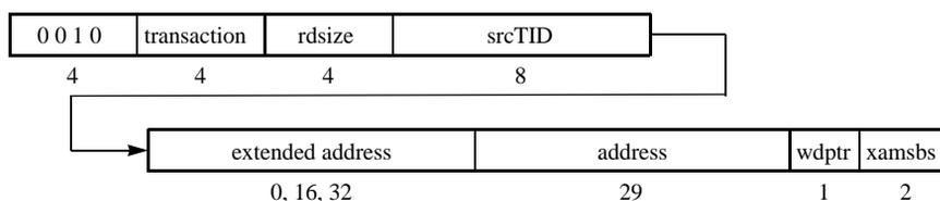
**Figure 4-2. Type 2 Packet Bit Stream Format**
