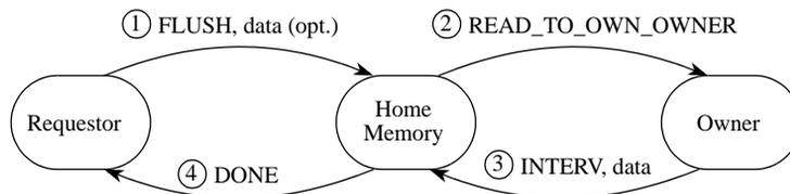
**Figure 3-20. Flush Operation to Remote Modified Coherence Granule**
