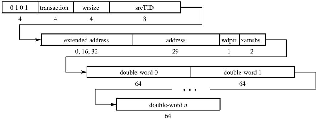
Figure 4-3. Type 5 Packet Bit Stream Format
