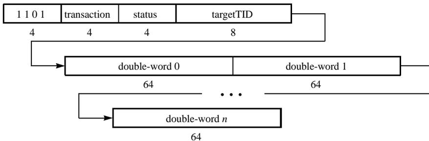
Figure 4-4. Type 13 Packet Bit Stream Format
