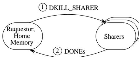
**Figure 3-21. Flush Operation to Local Shared Coherence Granule**
