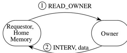
**Figure 3-3. Read Operation to Local Modified Coherence Granule**
