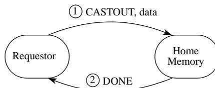
**Figure 3-14. Castout Operation on Remote Modified Coherence Granule**
