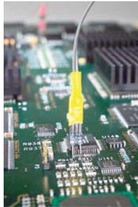
Figure 3: Flying lead set for high performance probing. (Photo courtesy of Agilent Technologies)
